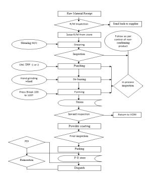
If these criteria's does not match the feedback is sent to the supplier. Inspection time per sheet: 5 minutes Shearing-type operations include:blanking,piercing,roll slitting, and trimming [7].
